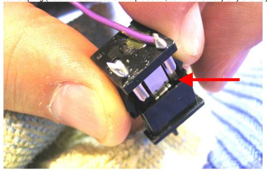
You will need to wriggle and adjust the two prongs that the wires solder to, to get them into the outside slot.
