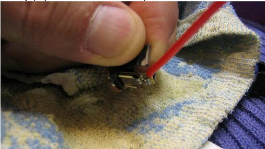
The switch should be wet from the contact cleaner.
