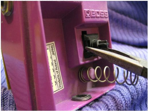
When the switch is released, pull it gently out of the pedal
