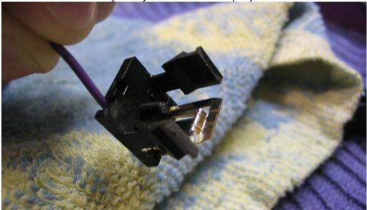
VERY carefully and gently, use a fingertip to open the switch contacts. Be careful to not touch the actual metal that meets to make the switch contact (tip of arrow).
